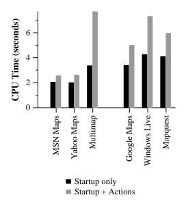
Figure 4: Computation time for 3 traditional map sites (left) and 3 interactive map sites (right). The black bars represent the CPU time required to load the site, and the gray bars represent the CPU time to load the site, zoom in twice, and move north once.
