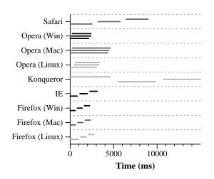
Figure 5: Concurrency behavior for popular web browsers. Each set of solid lines represents the execution of three frames loaded at the same time.
